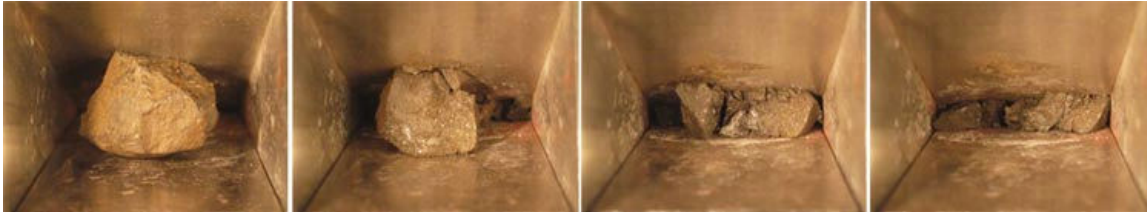
Caption: Looking down on the jaws of the Mars Rock Crusher, we see a magnetite rock get crushed into smaller and smaller particles.
